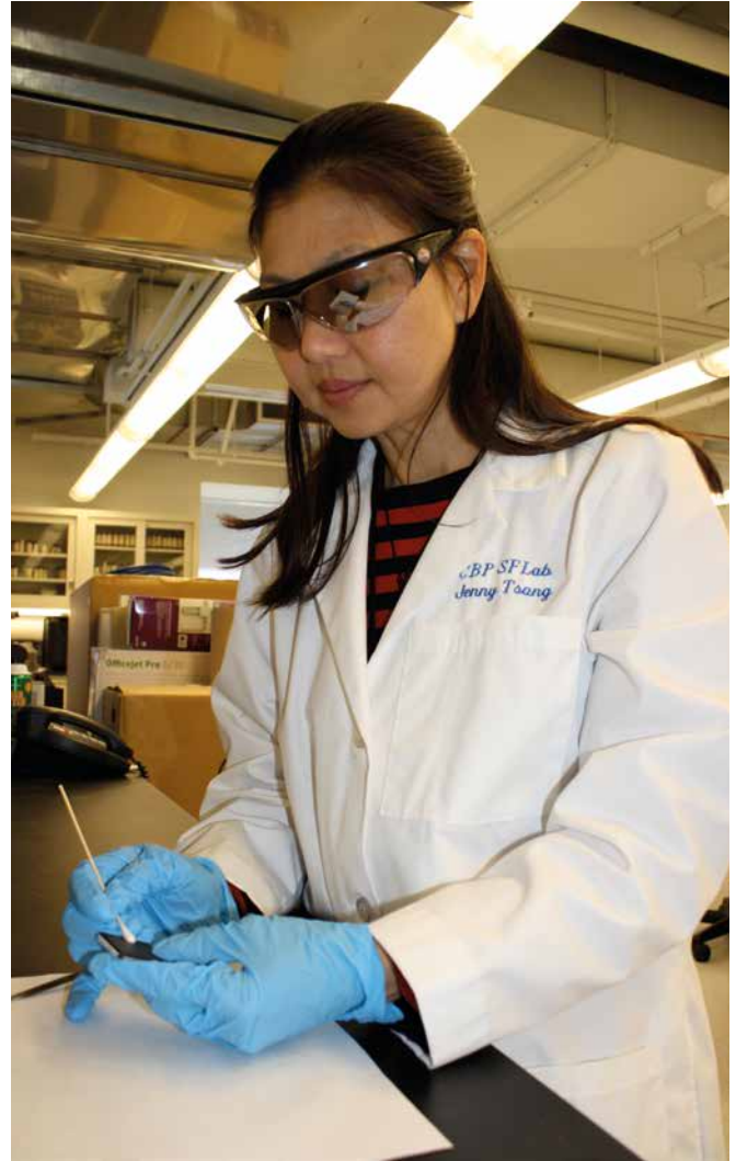
Jenny Tsang, Assistant Director of CBP's San Francisco laboratory, applies a chemical solvent to a computer chip to see if its coating or manufacturer's markings can be removed, one of the many signs of a counterfeit chip. Photo: Rand Careaga
