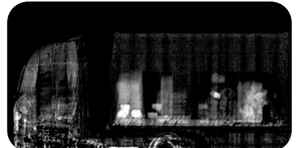
AXR-Wall Removal removes steel container walls from the X-ray image to highlight organic materials.
