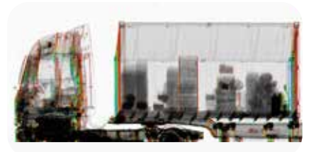
AXR-In Depth locates precisely objects across the entire width of the container.
