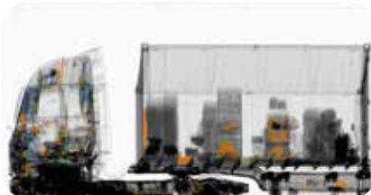
AXR-De-Overlapping identifies areas of interest to highlight concealed goods.
